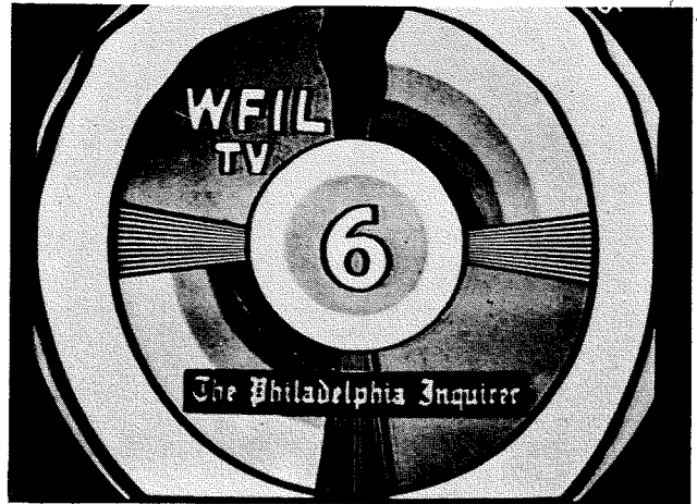
Fig. 4—"Hunting" due to improper control tube constants
