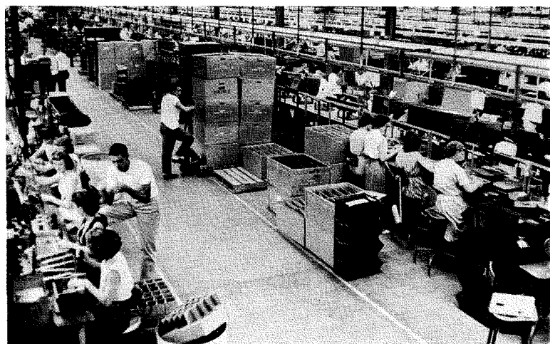
An overall view of the record-changer and amplifier assembly lines at RCA Victor's factory at Cambridge, Ohio. The plant, world's largest producer of packaged hi-fi instruments, has fifteen assembly lines capable of turning out 6,000 sets in an eight-hour shift. Inset is one of the instruments in RCA's complete hi-fi line.
